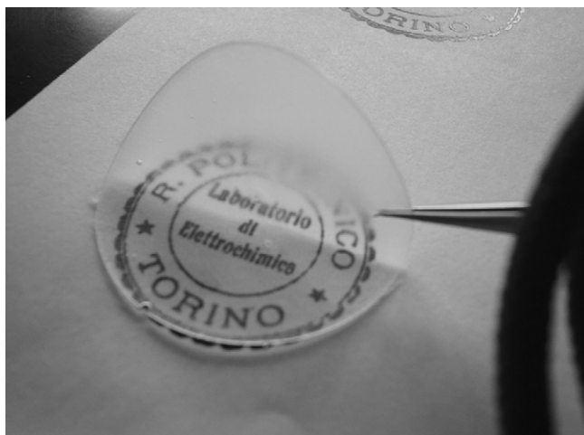
Fig. 2. Self-supporting polymer electrolyte membrane obtained by one-shot photo-polymerisation of the monomer BEMA with 60 wt.% of EMIPFSI and 10 wt.% of LiTFSI via UV irradiation (ILBM-60).
